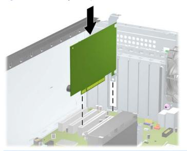
Figure 5-13 Installing an Expansion Card
